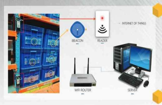
Smart Shelf System (Sistem Rak Pintar) able to give out location with accuracy level of 95% and 5% deviation as long as it is still in 1 row.
